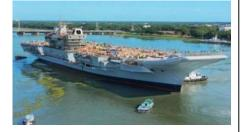
commissioned on (Independence Day) 15 August, 2022. The IAC has been constructed by Cochin Shipyard Limited (CSL). The IAC will use **ski-jump** technology for launching the aircraft from the carrier. It costs around **Rs 23,000 crore**. The IAC is 262 metres long, 62 metres wide and it has a height of 59 metres and it has over 2,300 compartments. The warship will operate MiG-29K fighter jets, Kamov-31 helicopters, and MH-60R multi-role helicopters.
